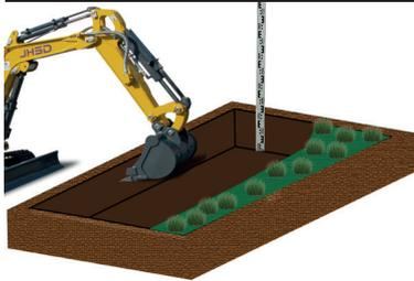
Excavate area for subbase to be installed. *For subbase calculation see overleaf.* Ensure to allow for: 10mm sand bedding layer; depth of grid and the 10-15mm dressing of aggregate when calculating depth from surrounding surfaces.
